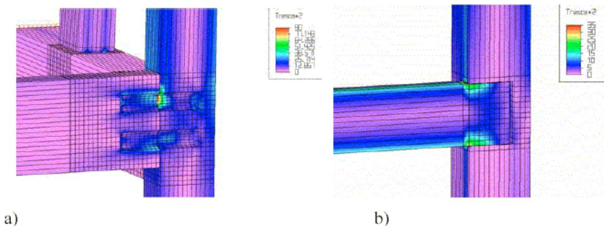
It is evident from the enclosed drawings that, in places showing the highest reduced stresses in cross sections of construction elements, the highest combined stresses in glue lines and joint elements were also generated.
