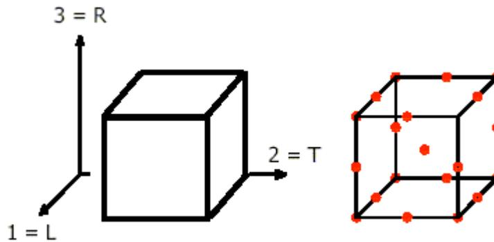
In the case of wood, which is an orthotropic material characterised by appropriate interrelationships between  $\varepsilon_L$ ,  $\varepsilon_T$ ,  $\varepsilon_R$  deformations and  $\sigma_L$ ,  $\sigma_T$ ,  $\sigma_R$  stresses, the following correlations were used for stress tensor:
