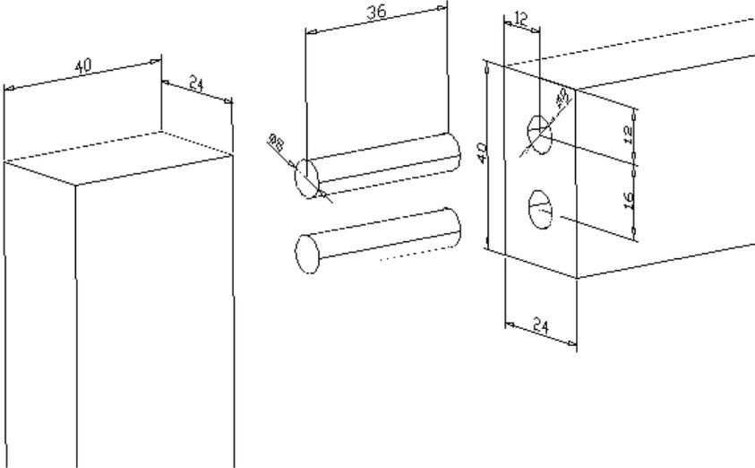
**Fig. 3. Dimensions of the connection with a tenon and mortise joint**
