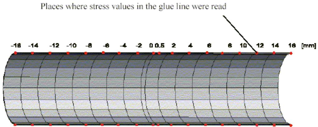
Fig. 10. The way stress values in the dowel were collected
