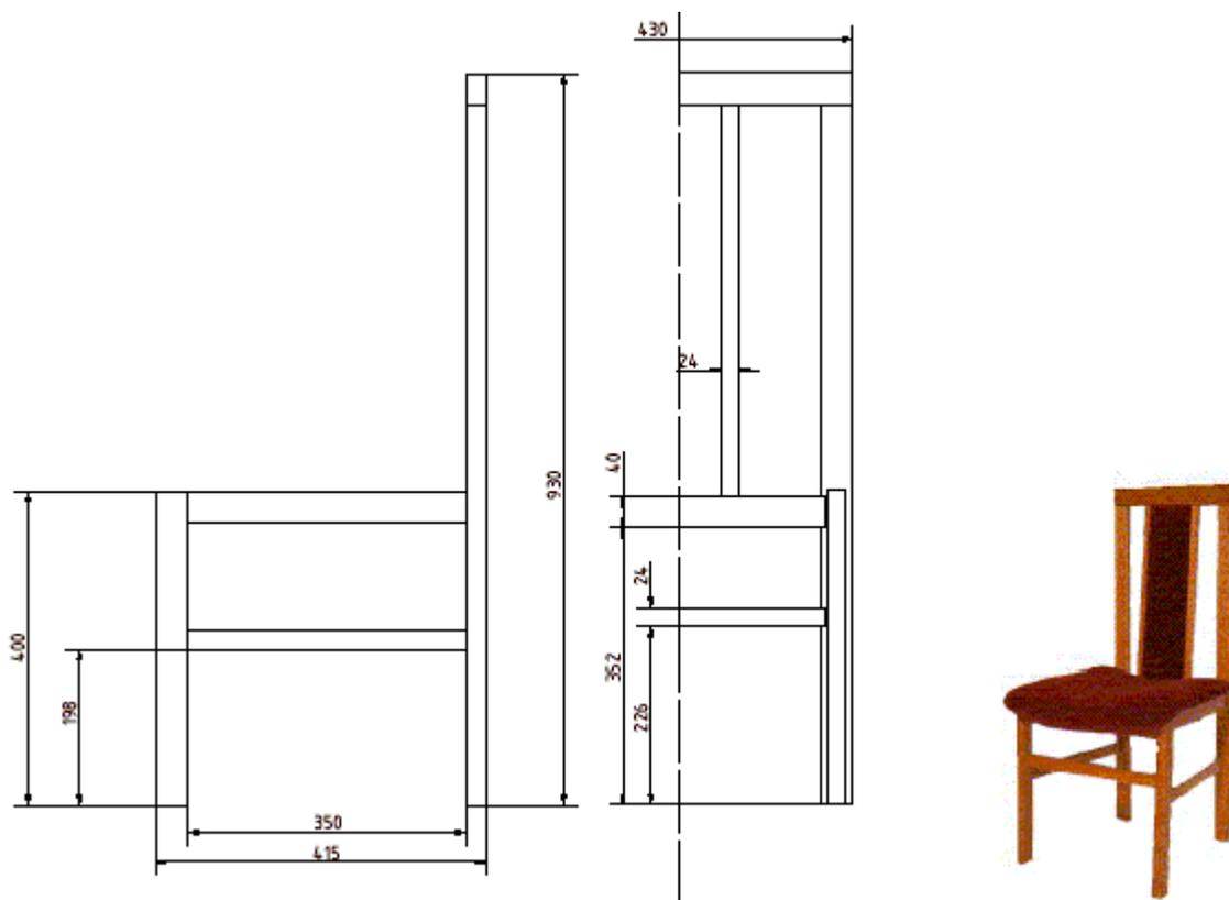
The basic constructional intersections of the examined piece of furniture were connections in a dowel joint (Fig. 2) used to connect legs and elements of the underframe and the backrest with the rear leg. Tenon and mortise joints (Fig. 3) were proposed to connect the bar and connectors with legs.
