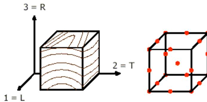
Fig. 8. Spatial isotropic element for glue line
