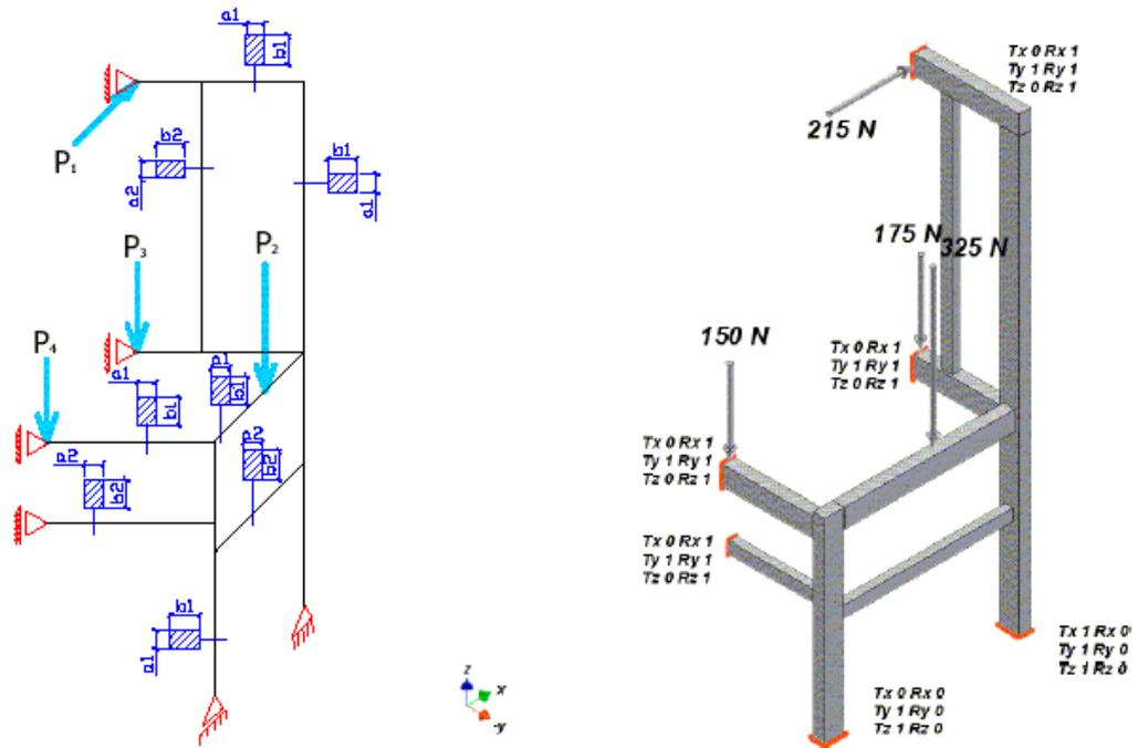
Spatial orthotropic elements from the 3D Continuum Elements containing 21 nodes (Fig. 7) were employed as calculating elements. On the other hand, glue lines were treated as isotropic material having the same deformation values in different directions (Fig. 8).
