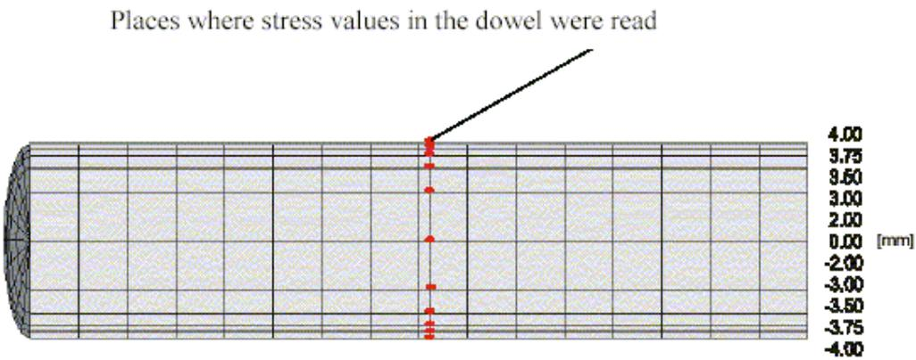
Fig. 11. The way stress values in the glue line of the tenon and mortise joint were collected
