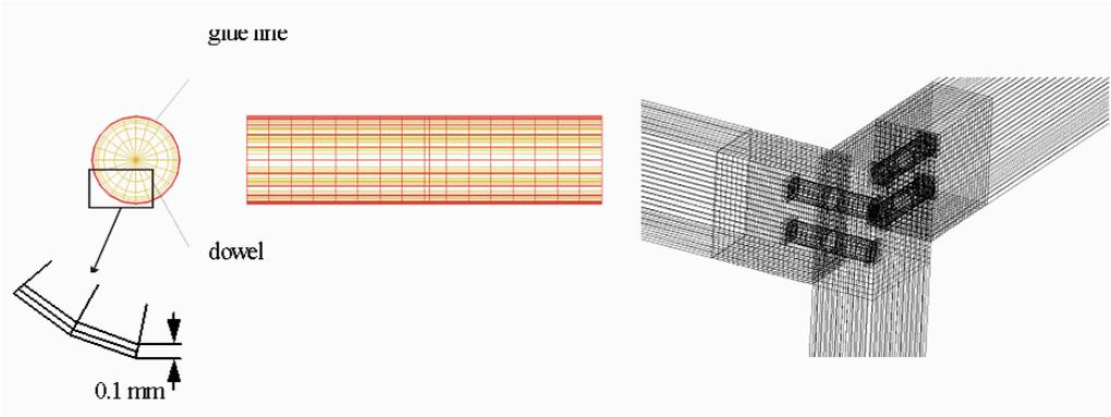
**Fig. 5. Network of finite elements for the tenon and glue line**
