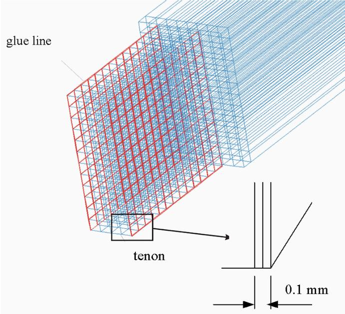
The strength analysis of the furniture construction was performed only for the symmetrical half of the spatial structure, loading it in accordance with the stipulations of the PN-ISO 7173:1994 standard (Fig. 6).
