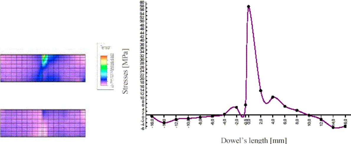
While evaluating the strength of furniture constructions, it is also essential to examine the state of tangential stresses in the joint material; this refers, in particular, to wood shear strength. Wood shear strength along its fibres was determined in the central part which is most exposed to damage (Fig.16). Distance from dowel axis.
