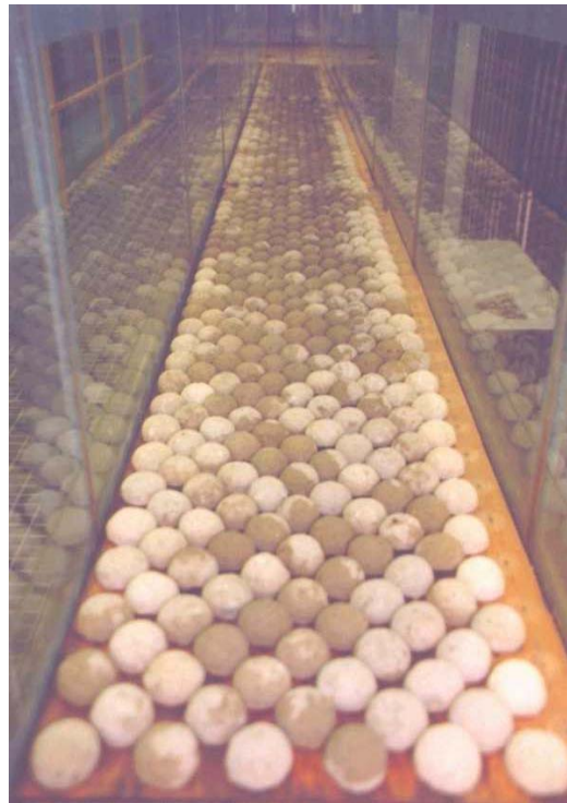
Fig.3. View of flume with artificial grains
