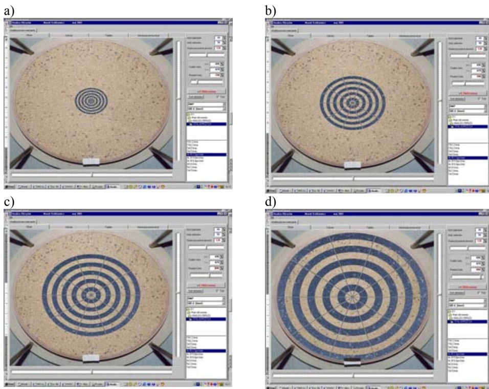
Fig. 6. Random mixing (determination of the analyzed surface for the variance estimation of the tracer's distribution; hundred-elemental net; radius lengths: a) r_1 = 100 pixels; b) r_2 = 200 pixels; c) r_3 = 300 pixels; d) r_5 = 460 pixels
