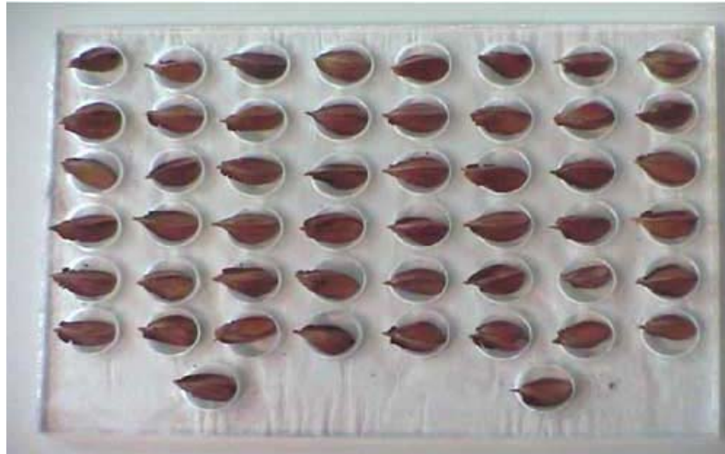
Figure 1. Beech seeds place in metaplex templed, prepared for vitality analyse by using X-ray radiography method
