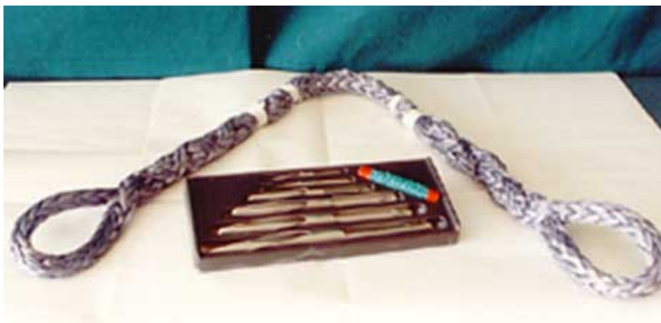
Fig. 1. A 10 mm diameter Dyneema SK60 strop, ready for tensile testing and a set of needles for intertwining
