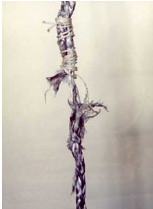
Fig. 3. The result of breaking a 10 mm Dyneema strop
