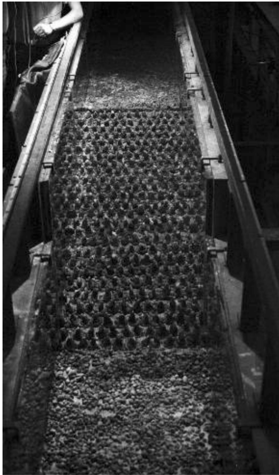
Phot. 1-3. RHS in the laboratory research site: RHS with stones arranged in a checker board pattern; experimental channel; flow over the sill and the stone-lined apron of the RHS.
