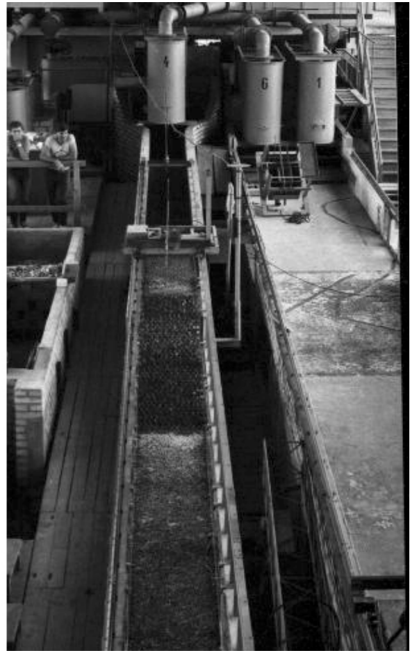
Phot. 1-3. RHS in the laboratory research site: RHS with stones arranged in a checker board pattern; experimental channel; flow over the sill and the stone-lined apron of the RHS.
