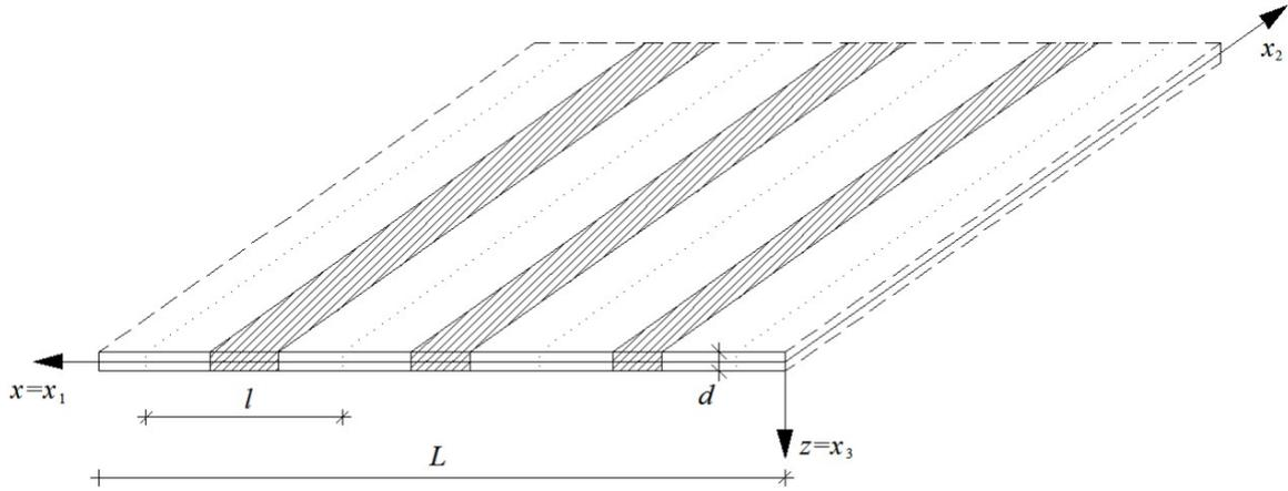
**Fig. 1. The fragment of a thin transversally graded plate band**
