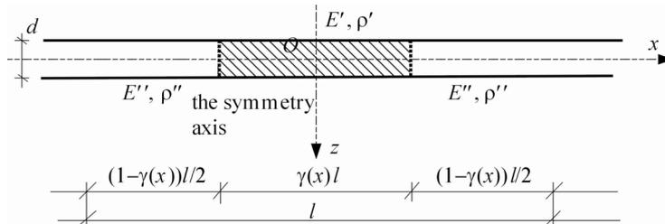
**Fig. 2. A cell of the transversally graded plate band**
