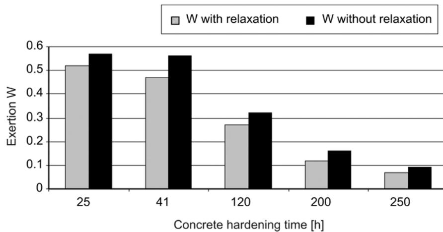
Fig. 16. Graph of the exertion function for HPC block ( $T_p = T_f = 20^\circ\text{C}$ ),  $W_{\max}$  after 41 hours
