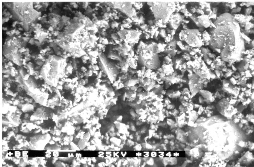
**Fig. 2. The microscopic picture (magnification  $\times 500$ ) of Silica Fume (own research)**
