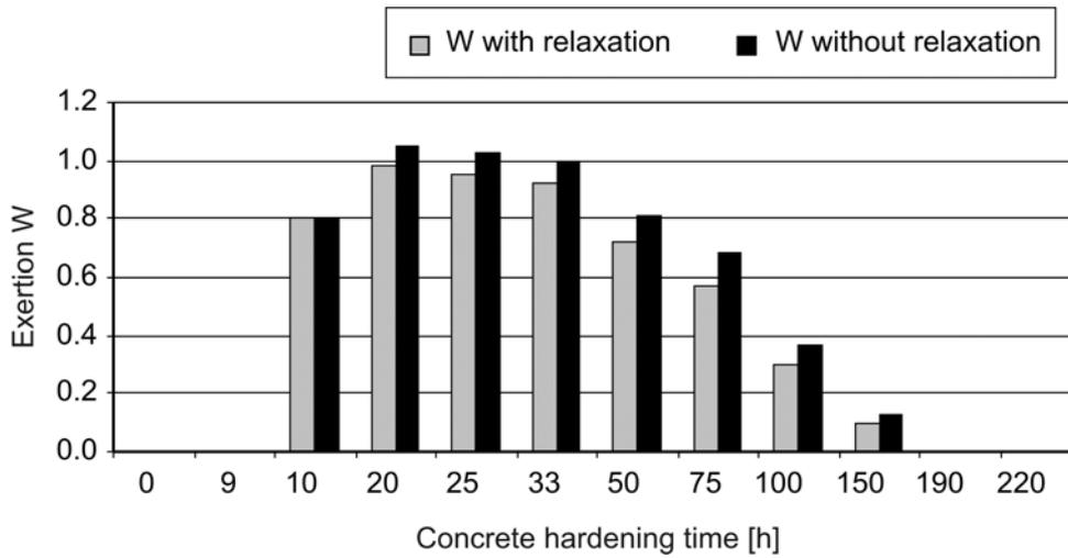
Fig. 13. Graph of the exertion on the external cylinder surface – function for OC
