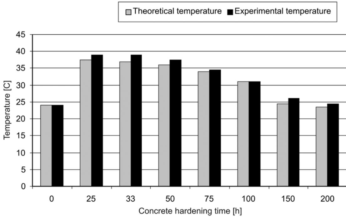
Fig 11. Surface temperature of hardening HPC block,  $T_{\max}$  after 33 h
