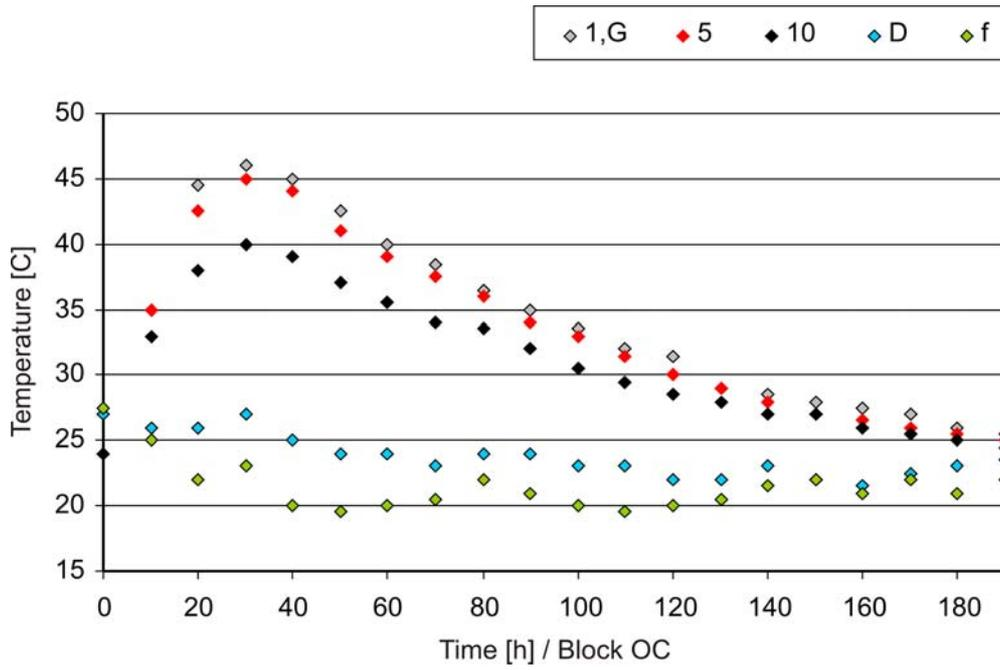
Fig. 9. Registered temperature distributions in the HPC block
