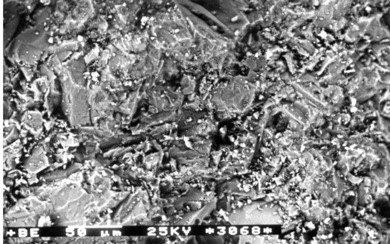
**Fig. 4. The microscopic picture (magnification  $\times 500$ ) of a hardened HPC cement paste (own research)**
