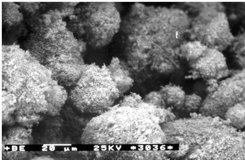
On Fig. 1 the microscopic picture of Bridge Cement 42,5 is presented and on the next one – Fig. 2 the microscopic picture of Silica Fume is presented as well. The different microstructure of these materials can be clearly seen. Cement grains are irregular but Silica Fume grains are fundamentally spherical.
